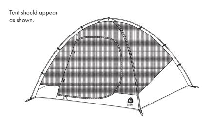
**STEP 7:** Unfold fly and place over tent so the zippered opening is located over the door.
