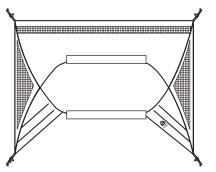
**STEP 2:** Stake the canopy to the ground by inserting stakes though the webbing loops at the side corners of the structure. Hammer the stakes into the ground at a 45° angle, making sure the sides are pulled out evenly.
