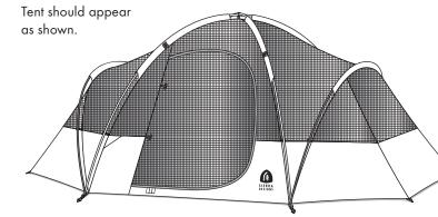
**STEP 8:** Unfold fly and place over tent so the large zippered vestibule is located over mesh door and pole sleeve is located over the doors. Make sure seams of fly align with tent poles. Fasten the hook and loop fasteners on the underside of the fly to the fiberglass poles at all locations.
